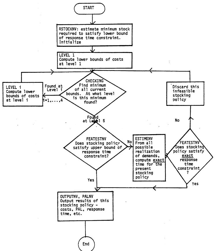
\*Flowchart for Vanning is identical with "NV" functions replaced by corresponding "V" functions.
