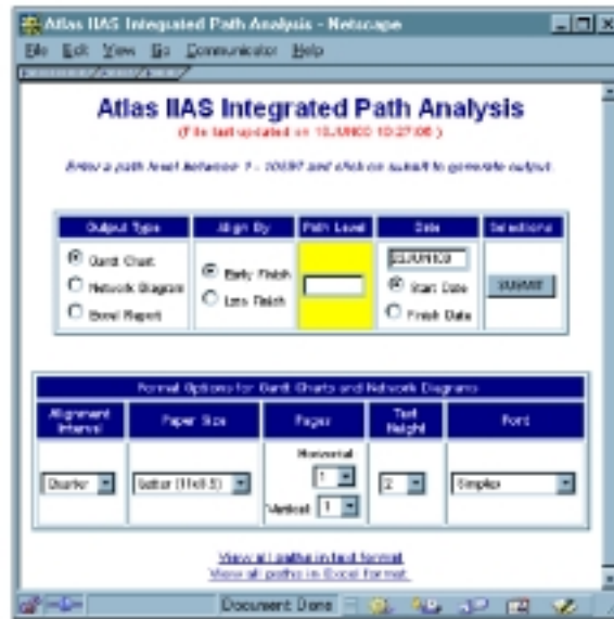
Figure 12: This Web page drives the Atlas II cycle-time reduction application. The user chooses the chart type, schedule type, path level (longest path) to find, date information, and information for the desired chart format.
