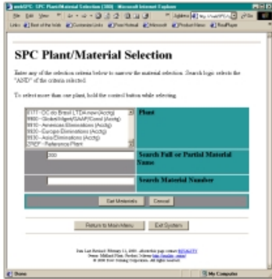
Figure 9: This Web page is the entry point for the Dow Corning SPC application for producing statistical process control charts. The user can select a plant and a search string to locate the types of materials made at that plant.
