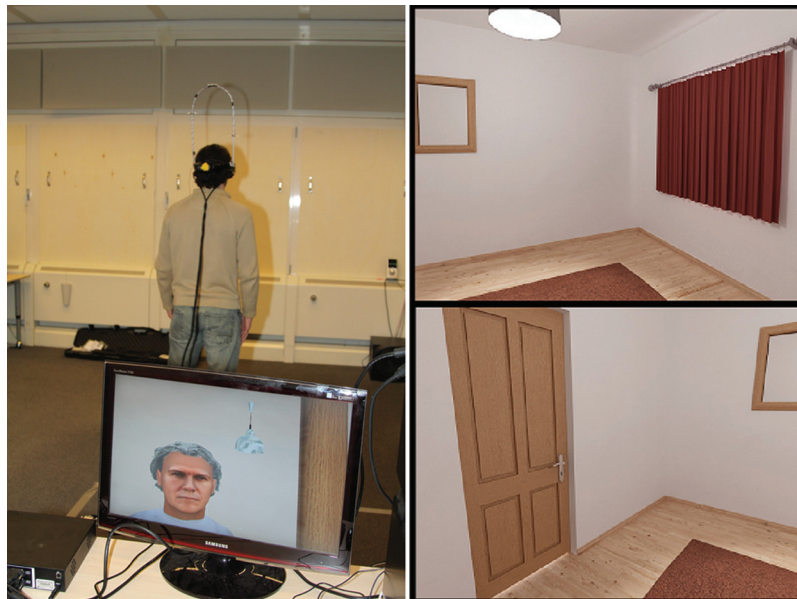
Fig. 1. Illustration of the virtual reality setup in Study 2. In the photo on the left, a participant is wearing the head-mounted display in the immersive virtual reality room; the computer screen at the bottom shows the age-progressed version of himself that the participant is seeing through the display. The images on the right show the virtual room.
